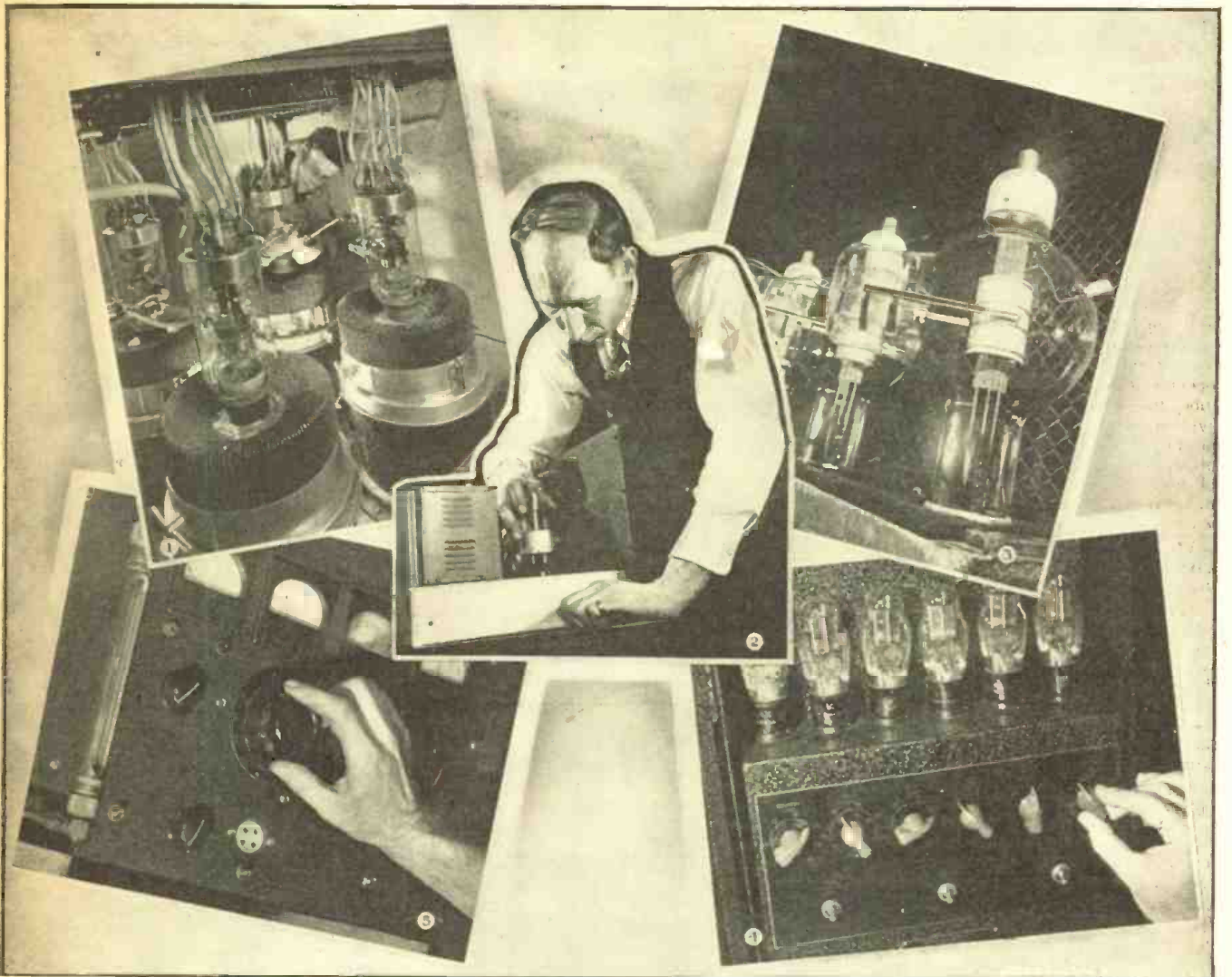
Symbols of modern radio and industry! Photo (1) shows four of the big air-cooled 50,000-watt modulating tubes used in a large broadcasting station. Two of these are spares or "standbys." Simply by pushing a button the operator can put them into service without removing defective tubes or interrupting the transmission. The center photo (2) shows the special moisture-defecting tube going into place in an electronic installation for control of moisture in a manufacturing process. The photo at the upper right (3) shows U.H.F. tubes used in inter-continental communications. Photo at the lower right (4) gives some idea of the appearance of a precision electronic timer, which automatically divides the time required for a spot-weld, into fractions of a second. Photo (5) shows the hand of an operator setting the adjustments on an electronic furnace control, which provides high efficiency, not obtainable by other means.
